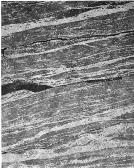
A. THE "STRINGER LEAD" TYPE OF VEIN, SHOWING STRINGERS AND SEAMS OF QUARTZ AND ORE IN A SCHISTOSE COUNTRY ROCK. THIS IS A PHOTOGRAPH OF A POLISHED SECTION OF THE VEIN IN THE GOLD HILL MINE. THE EMMONS VEIN IS VERY SIMILAR.
